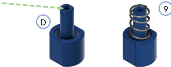
12. - You can test the locking mechanism in the body by placing the spring inside the button, placing the button into the hole and compressing the spring until the top of the shaft protrudes through the top of the body. There should be little to no resistance. If there is, remove the button and lightly sand the button shaft and the inside of the hole.
