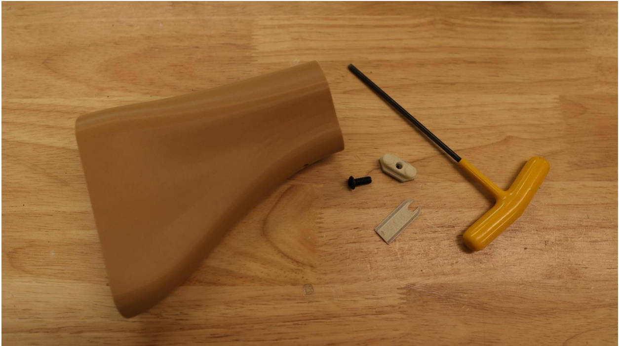
Figure 9 Parts needed for the retention mechanism.
