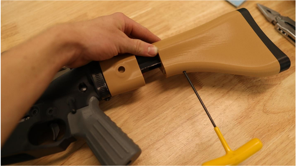
Figure 25 Feeling for the detents by sliding the butt back and forth while tightening the block.
