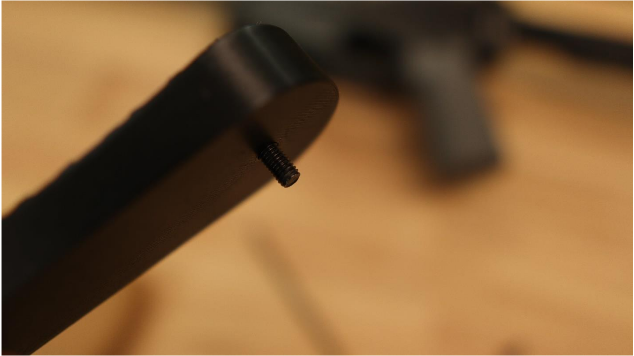
Figure 20 Push the screw through the plate, and then fasten it to the stock.
