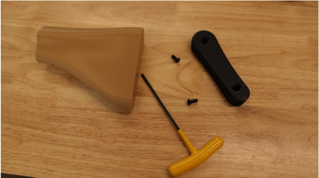
Figure 18 Parts needed to install the pad.
