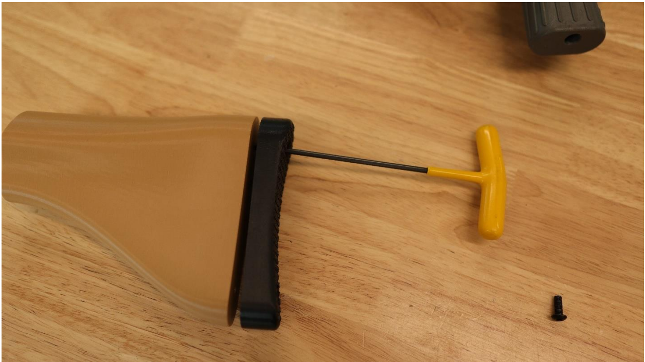
Figure 21 Add one screw and then the other.
