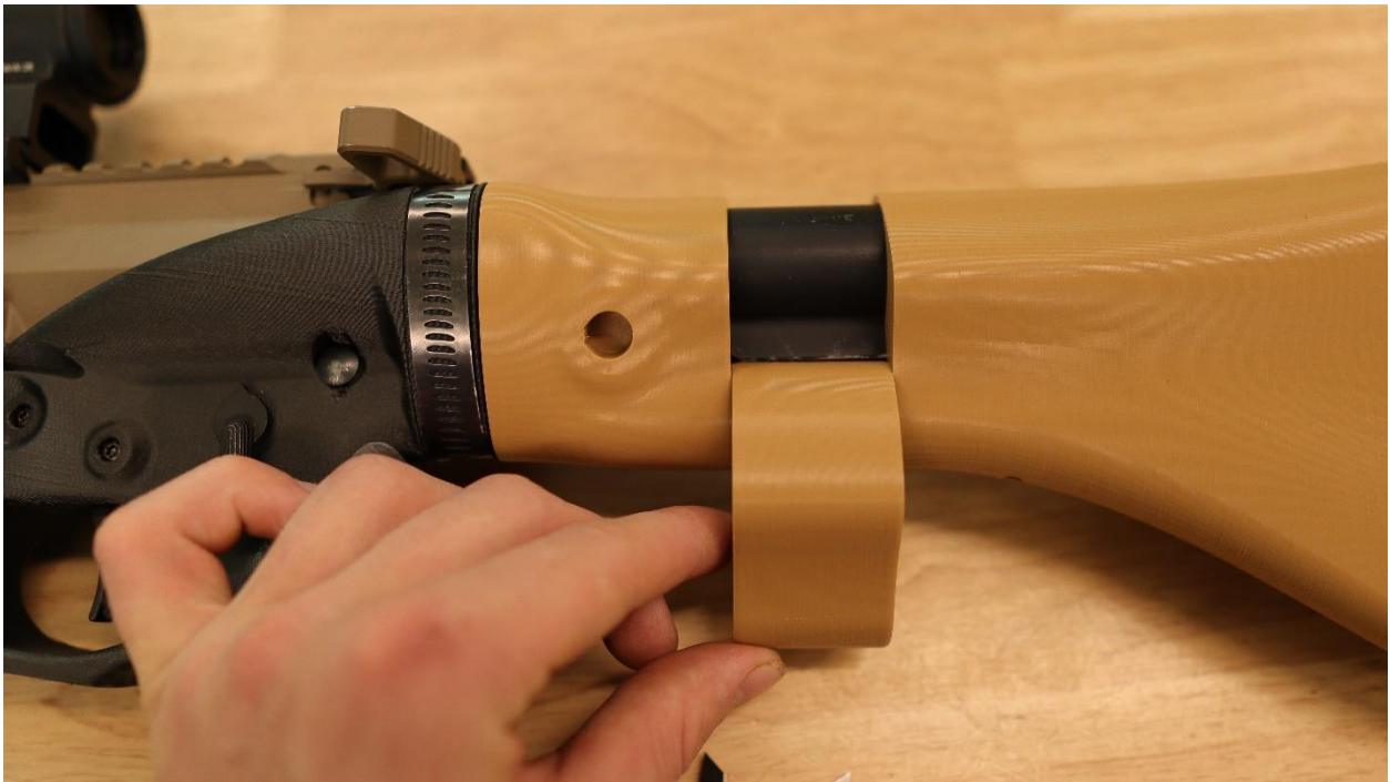
Figure 26 If you have already printed the neck, simply slide the stock up to the neck and torque the screw.
