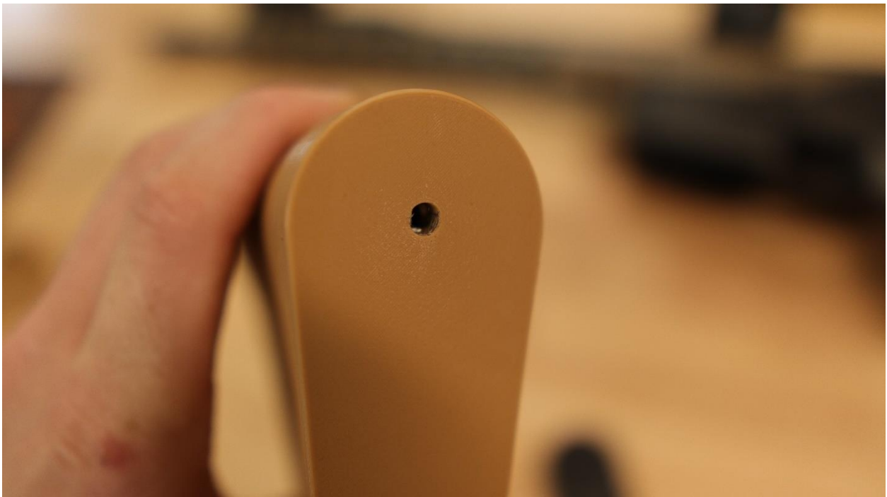
Figure 19 The holes have flats on each side, this is to act as a lock nut and prevent screws from backing out.
