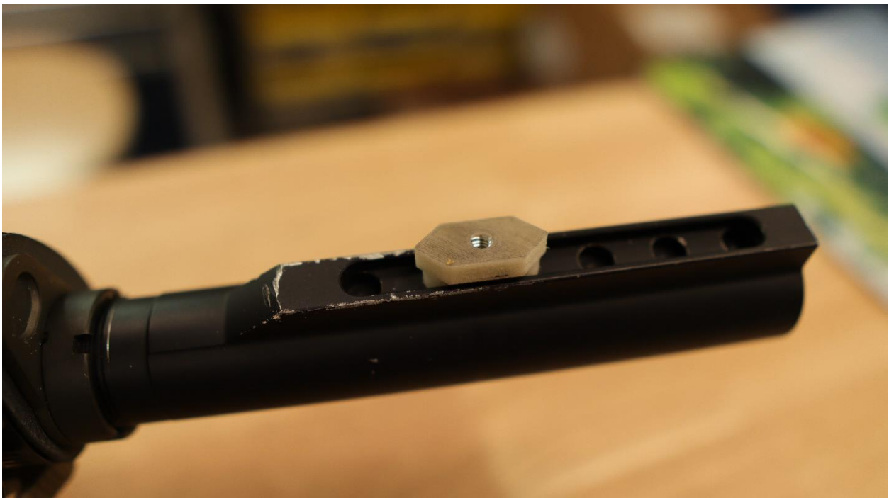
Figure 10 How the block interacts with the buffer tube.
